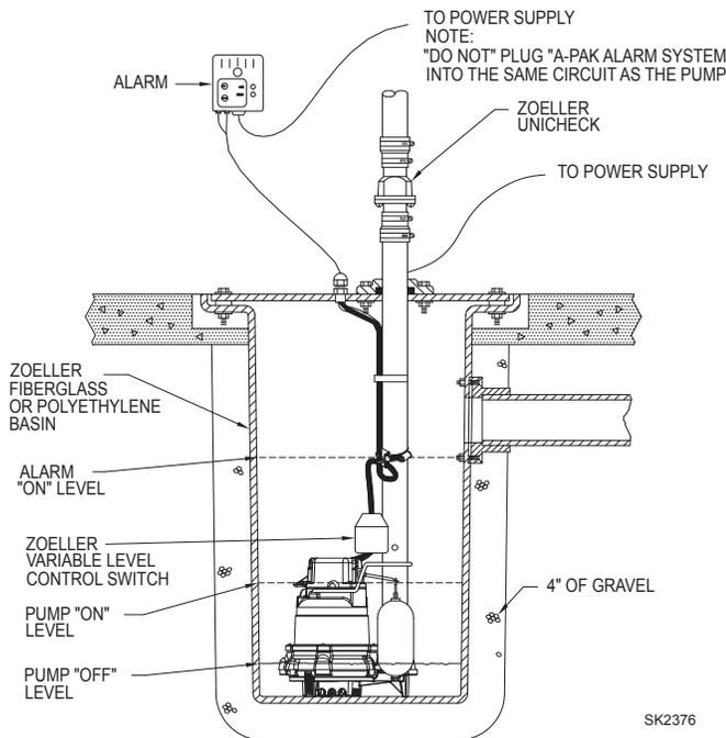
High water alarms provide the owner with early notification that the water level is continuing to rise in the application. This could be due to a pump failure or power outage, or the pump is simply overwhelmed in the application.
