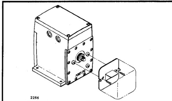
FIG. 1—MOUNTING THE Q181 ON M944 AND M945 STYLE MODUTROL MOTOR, OR ANY MOTOR WITH BOSSES.
