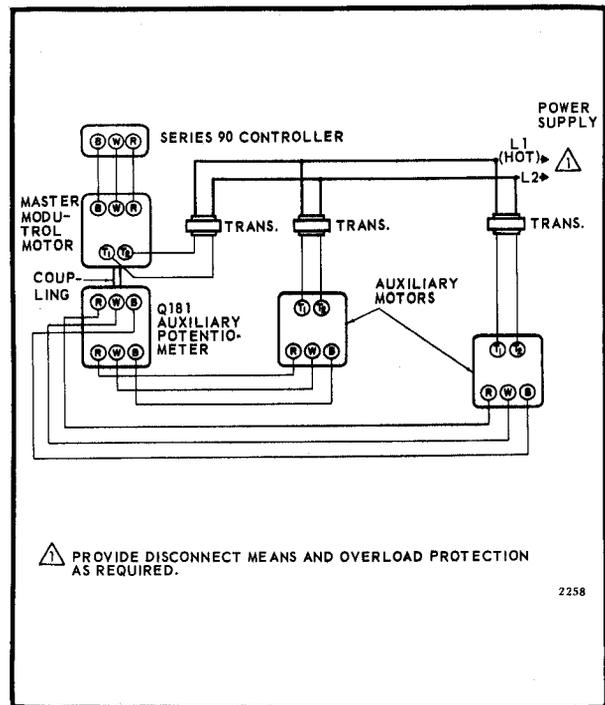
FIG. 4—TYPICAL HOOKUP OF Q181, TWO POTENTIOMETER MODEL, AND TWO AUXILIARY MOTORS.
