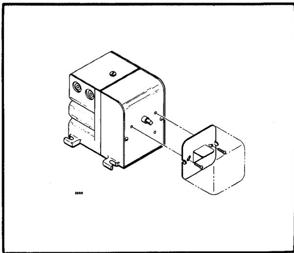
FIG. 2—MOUNTING THE Q181 ON THE M934.
