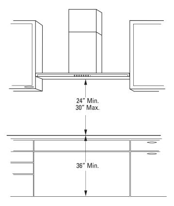
The vent hood must be installed 24" min. and 30" max. above the cooking surface. The hood installation height, from the cooking surface to the bottom of the hood, depends upon ceiling height.
