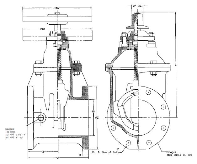
\* Face to face dimensions (inch) conform to ASME B16.10
