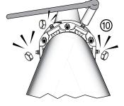
Step 11 • Pressure test for leaks before backfilling.
