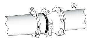
**Step 7** • The pipe should be centered such that the space between the OD of the pipe and the ID of the RFCA is even all around the pipe. Slide the RFCA gasket into position with the beveled edge engaging the beveled end of the RFCA body.
