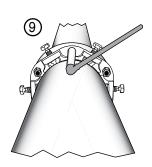
Step 10 • Hand tighten the restraining bolts in the clockwise direction until the lugs touch the pipe. Continue to tighten in a uniform criss-cross pattern until the heads break off.
