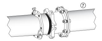
Step 8 • Slide the RomaGrip toward the RFCA body until the nose of the gland touches the gasket. Insert the T-bolts and hand tighten the nuts. Make any deflection after hand tightening the T-bolt nuts but before tightening them to the proper torque specifications.
