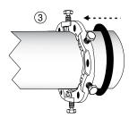
**Step 4** • Place the RomaGrip gland on the pipe with the nose extension towards the plain end.
