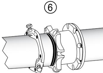
**Step 7** • The pipe should be centered such that the space between the OD of the pipe and the ID of the RFCA is even all around the pipe. Slide the RFCA gasket into position with the beveled edge engaging the beveled end of the RFCA body.
