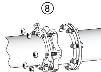
**Step 9** • Tighten T-bolts evenly, alternating to diametrically opposite position at approximately 20 ft-lbs increments to the recommended torque for your size RFCA.
