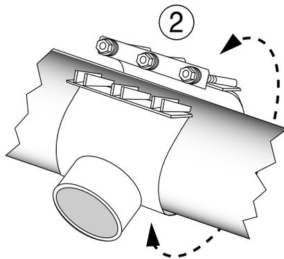
**NOTE:** For larger sizes, it may be necessary to remove the spring washer so that the lifter bar can snap into place over the sidebar edge. In this event, after removing the spring washers, replace two of the nuts and snap lifter bar in place as per the instructions. Tighten the two nuts until the third bolt has room to install the spring washers and nut, tighten the third nut until the other two bolts have room for the spring washer and nuts and finish tightening per instructions.
