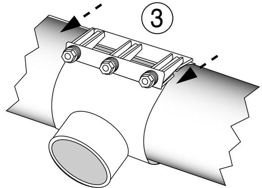
**Step 4** • Tighten all nuts evenly in 20 ft-lbs. increments to a minimum of 40 ft-lbs. Use a wrench with at least a 12 inch handle. Branch connections can be made with conventional coupling devices depending on branch material.
