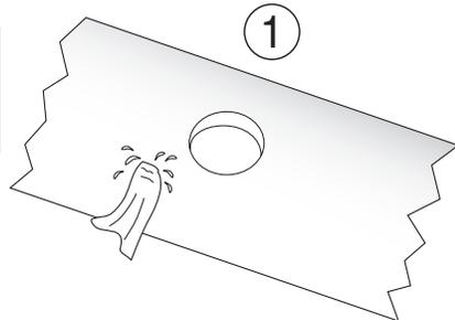
**Step 2** • Back off nut to the end of the bolt – DO NOT REMOVE. Separate the ends of the saddle and position the branch over the hole that had already been cut in the pipe (see Step 1).
