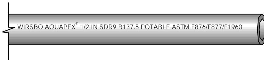
AQUAPEX® is rated at 160 psi @ 73.4°F, 100 psi @ 180°F and 80 psi @ 200°F. These pressure and temperature ratings are issued by the Hydrostatic Design Stress Board of the Plastic Pipe Institute (PPI). PPI is a division of the Society of Plastics Industry (SPI).
