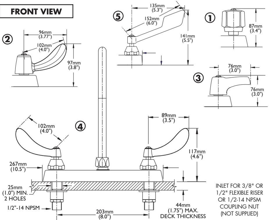
INLET for 3/8" OR 1/2" FLEXIBLE RISER OR 1/2-14 NPSM COUPLING NUT (NOT SUPPLIED)
