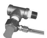
The Victaulic® Series 749 Auto Drain is used in Series 756 Dry and Series 758 Actuated valves that have either a Series 753/753-A Dry Actuator or a Normally Closed solenoid valve. Once tripped, the Auto Drain constantly drains the piston charge line, preventing the piston from repressurizing. The Auto Drain remains open until it is manually reset during the valve resetting procedure.
