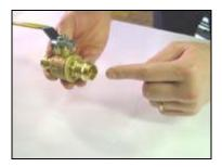
C. Check seal for correct fit. Do not use oils or lubricants. Use only the valve's yellow NBR o-ring seals.
