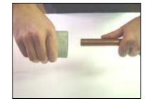
B. De-burr tubing on the inside and outside to prevent cutting of the valve's o-ring seals.
