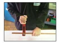
A. Cut copper tubing at right angles (using displacement type cutter or fine-toothed steel saw).
