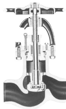
**Angle valves** are otherwise similar to conventional globe valves, but the less tortuous flow path yields lower pressure drop. Angle valves are particularly economical in piping layouts where use of this configuration eliminates an elbow and associated flanged or welded joints.
