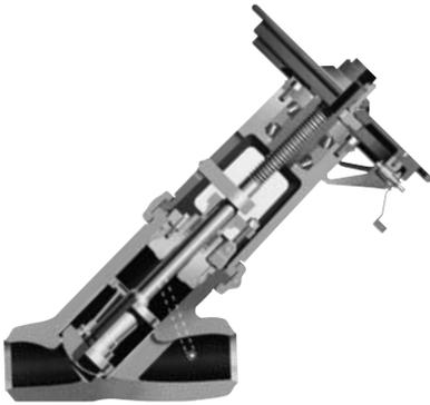
• **Seats** – Industrial globe valves are available from various manufacturers with a broad variety of seat designs — flat or tapered, and integral or inserted (threaded or welded).
