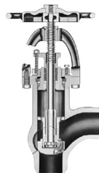
**Inclined bonnet or “Y type” valves**, such as Univalves® and Flite-Flow® valves, yield lower pressure drop than other styles, because they permit a more nearly straight-through flow path. Typically, they require a longer stem travel. In large sizes, this body shape is heavier and requires a greater end-to-end length than conventional globe valves.
