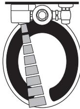
2. As the user enters the beam's effective range, 8" to 54" (203 mm - 1372 mm), the Object Lock Infrared Sensor senses the user.
