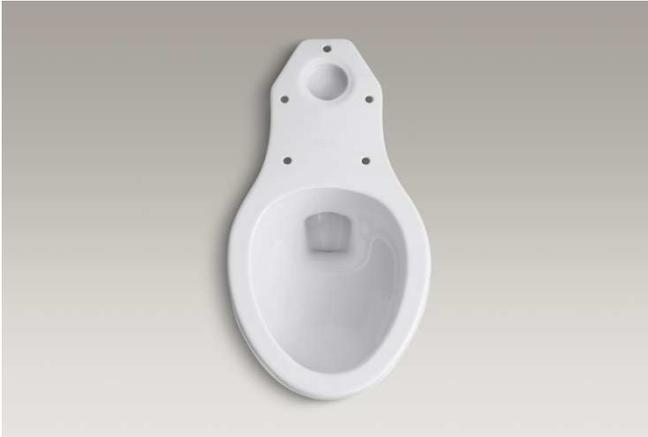
The elongated bowl toilet shall be made of vitreous china. Toilet shall be 30-1/8" (765 mm) in length, 21-1/4" (540 mm) in width, and 31-1/4" (794 mm) in height with an 11-1/2" (292 mm) by 9-1/2" (241 mm) water area. Toilet shall be 12" (305 mm) rough-in. Toilet shall feature 2-1/4" (57 mm) glazed trapway. Toilet shall be less seat and supply.
