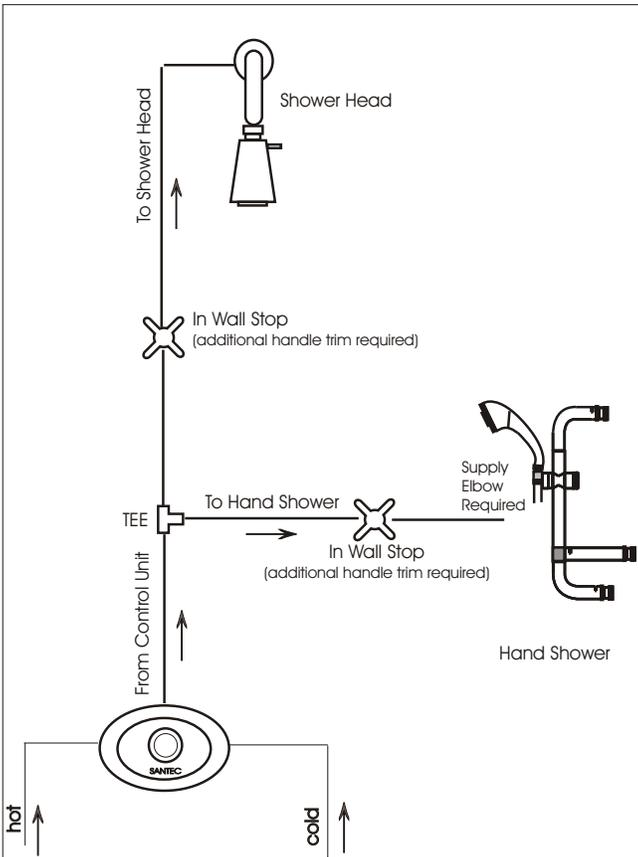
1. Using 1/2" or 3/4" IPS, plumb the stop valve accordingly to the handle styles described below. (Measurement is from the center of water connection to outside of finished wall).
