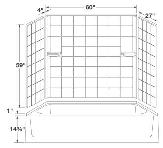
General: Furnish and install as shown on plans, E. L. Mustee & Sons, Inc. Tub/Shower TOPAZ™ Combination Units, semi-gloss, three piece fiberglass wall system and fiberglass bathtub 30" x 60" left for right-hand drain. Construction on units shall be modled reinforced fiberglass using matched metal molds under extreme heat and pressure creating a uniform thinkness. Shall meet ANSI Specification Z 124-2017. Color: \_\_ \_\_\_\_ (White, Bone, Biscuit). Install in compliance with local codes.
