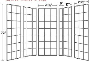
General: Furnish and install as shown on plans, fiberglass VARISTONE™ Shower / Bathtub Walls Model 572T as manufactured by E. L. Mustee & Sons, inc. Shall be semi-gloss, 5-piece wall system. Panels are molded using matched metal molds under extreme heat and pressure with a minimum thickness of 125 mils. Shall meet ANSI Specifications Z 124-2017 Colors: \_\_\_\_\_\_ (White, Bone)
