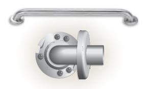
TWIST-LOCK CONCEALED FLANGE — locking tabs on the flange cover plate. Turn 15 degrees under the matching wedges on the mounting flange.
