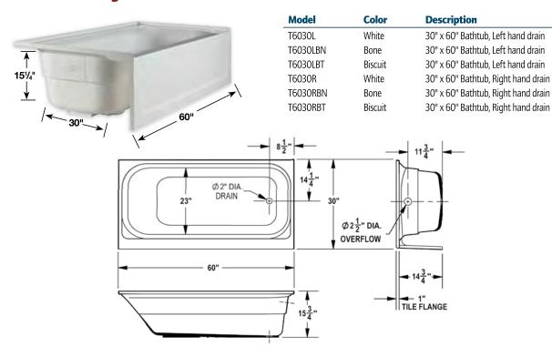
**General:** Furnish and install as shown on plans, E.L. Mustee & Sons, Inc. TOPAZ™ Fiberglass Bathtub 30" x 60" right or left-handed Model: \_\_\_\_\_\_. Construction shall be molded, reinforced fiberglass using matched metal molds under extreme heat and pressure. Shall meet ANSI Specification Z 124-2017. Color: \_\_\_\_\_\_ (White, Bone Biscuit). Install in compliance with local codes.
