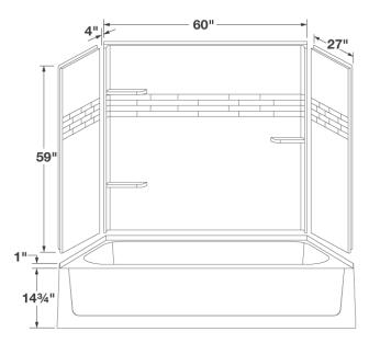
**General:** Furnish and install as shown on plans, E. L. Mustee & Sons, Inc. 680 TOPAZ<sup>™</sup> bathtub walls semi-gloss, three-piece wall system and TOPAZ<sup>™</sup> Fiberglass Bathtub 30" x 60" right or left-handed drain. Construction shall be molded, reinforced fiberglass using matched metal models under extreme heat and pressure with a uniform thickness. Shall meet ANSI Specification Z 124-2011. Color: White. Install in compliance with local codes.
