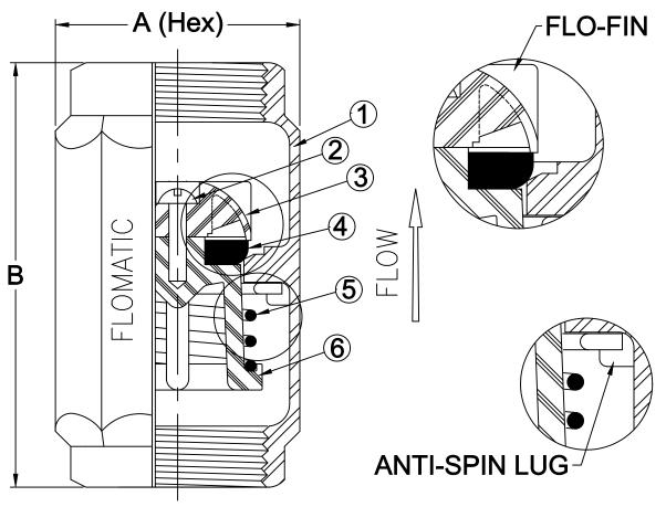
Temp Max: 180°F (80°C) Pressure Max: 400 psi (2758 kPa)
