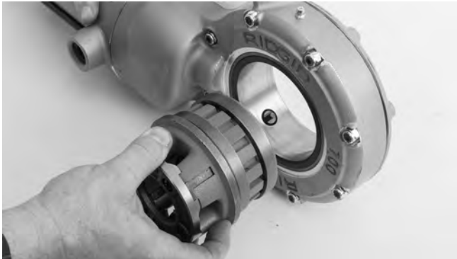
Figure 4 – Installing Die Heads into 700 Power Drive
