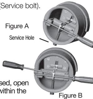
3. Locate the service hole and thread in the service bolt by hand until it contacts the linkage. (Figure A)
