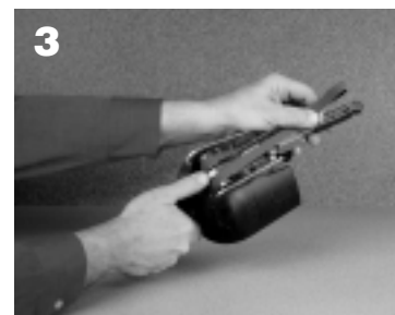
3 Depress idler arm lever and pull belt toward the contact wheel.
