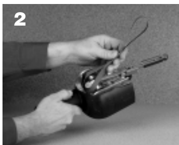
2 Form a loop in belt keeping the belt splice between fingers as shown in photo above. Slip lower loop of belt under the drive wheel.
