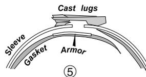
**Step 6** • Begin by tightening the center bolt, and work toward each end, tightening all nuts evenly in 20 ft-lb. increments. On clamps with more than one section, maintain equal gaps between sections, keeping torques as evenly balanced as possible. Use a wrench with at least a 12" handle.
