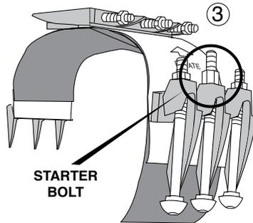
**Step 4** • Wrap the clamp around the pipe and snap the starter bolt head(s) into the open lug(s). Tighten until the other bolts can be snapped into the lugs.
