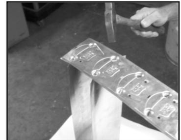
5. Align the vanes on the second length of rail and hammer over the vane, securing it to the rail.
