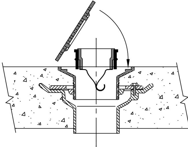
THE 3" TRAP GUARD COMES INSIDE A FLEXIBLE BUSHING THAT WILL FIT MOST 3-1/2" STRAINER TAILPIECES OR ANY 3" HUB SIZE OPENINGS, PLASTIC OR CAST IRON.
