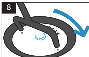
8 Insert new cartridge into housing and turn key to right to lock and click into place.
