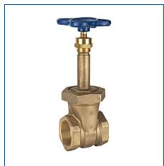
**Specifications UPC** Code 039923618290 Gate Valve Type **Valve Size** 1/4 in Material **BRZ Cast Bronze Description** T134 1/4 THD 150# RS GATE BRZ Multi-Turn **Turns / Operation** Seat / Seal Material **Bronze Connection Type** T -- Female NPT Thread (FIPT) Valve Gate Stem Design RS - Rising Stem Valve Multi-Turn Bonnet Design Union Bonnet Standard Handwheel **Operation Type**
