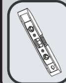
**3** If mounting directly to wood stud, Plastic Anchors are not required. If mounting to drywall or tile, select appropriate 1/4" drill bit and drill guide holes at marked locations.
