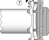
**Step 7** • Install T-bolts in the MJ fitting and gland. Tighten hand tight.
