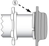
GripRing up the pipe until its face is flush against the MJ gasket. For best results, orient the gap in the GripRing in the down position.
