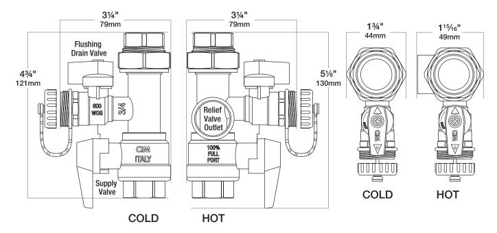
All valve kits include integrated union adapters for direct connection to cold water inlet and hot water outlet of the tankless water heater. Valve kits include integrated full port supply valves and full port system flushing/drain valves with linked cap. \*Hot water valve assembly includes outlet access port for included (unless otherwise noted) ASME rated 150 PSI relief valve.
