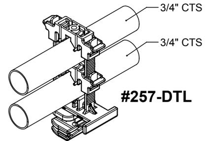
The HOLDRITE® Strut Clamp™ #257, #257-DT & #257-DTL is a strong variable closure clamp. Clamp supports up to 1" CTS tubing sizes. Supports Copper, PEX, CPVC tubing, conduit, etc. Framework complies with UL94V-2 fire rating.
