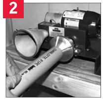
• Chamfer (bevel) the end of the pipe  $10^{\circ}$   $-15^{\circ}$ .
