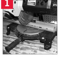
Acceptable tools include miter saw, reciprocation saw, and mechanical cut-off saw with
