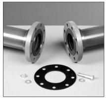
conveyed in the piping system. A gasket 1/8'' thick with a Durometer, scale "A", hardness of 55 -80 is normally satisfactory.
