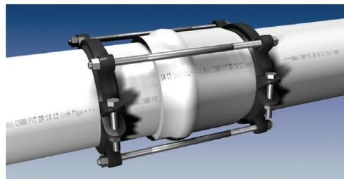
5. Install both halves of the restraint ring at the proper location, tapping each half into place. Make sure that the complete ID of the ring is touching the pipe before installing the side bolts. Tighten the side bolts evenly to 60 ft-lbs torque (110 ft-lbs on 8 inch, 10 inch and 12 inch).
