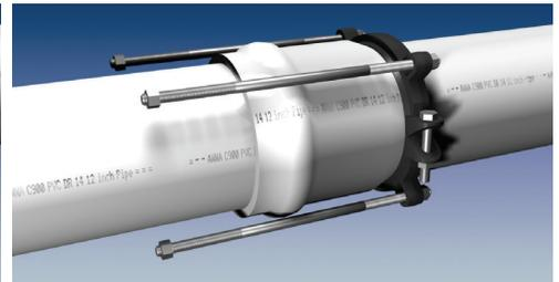
The Series 1600TD is designed for restraining ductile iron pipe and C900 PVC at push-on bell joints. It has a split, serrated restraint ring with heat treated inserts on the spigot and a split non-serrated ring behind the bell.
