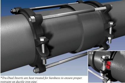
\*\*Two inserts are located near the clamp points on each half of the split serrated ring. This design provides maximum restraint on both ductile iron pipe and C900 PVC pipe enabling the product to be truly Tru-Dual.
