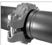
**5. ASSEMBLE JOINT:** Assemble the joint by inserting the grooved end of a mating component into each opening of the coupling. The grooved mating component ends shall be inserted into the coupling until contact with the center leg of the gasket occurs.
