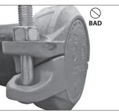
BAD ASSEMBLY (BOLT PADS ARE NOT IN METAL-TO-METAL CONTACT)
