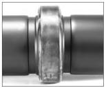
7. JOIN MATING COMPONENTS: Align the centerlines of the two grooved mating component ends. Slide the gasket into position and center it between the groove of each mating component.
