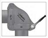
**6. COMPLETELY TIGHTEN NUT AT SECOND OUTSIDE LOCATION:** Completely tighten the nut at the second outside location until metal-to-metal contact occurs at the bolt pads. Verify that the fitting's keys still engage the grooves completely and that the oval neck of the bolt seats properly in the bolt hole.
