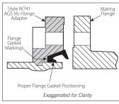
**5. POSITION AND INSTALL FLANGE GASKET:** Verify that the Flange Gasket is positioned properly, then install the Flange Gasket into the gasket pocket (cavity between the pipe OD and flange recess). The Flange Gasket shall always be assembled with the color-coded lip on the pipe and the other lip facing the mating flange. When installed correctly, the lettering on the Flange Gasket will not be visible when viewing the face of the Style W741.
