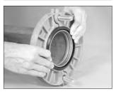
**7c.** Verify that the Flange Gasket is still seated properly within the gasket pocket of the Style 441 and that the lettering on the Flange Gasket is not visible when viewing the face of the Style 441.
