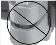
5. Visually inspect each bolt pad location at every joint to verify that metal-to-metal contact is achieved across the entire bolt pad section.
