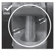
PROPERLY ASSEMBLED JOINT **BOLT PADS WITH EQUAL, POSITIVE** OFFSETS AT THE BOLT PADS
