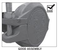
(END CAP IS SEATED WITHIN THE COUPLING WITH THE CORRECT SIDE FACING OUT AND COUPLING BOLT PADS ARE IN METAL-TO-METAL CONTACT)
