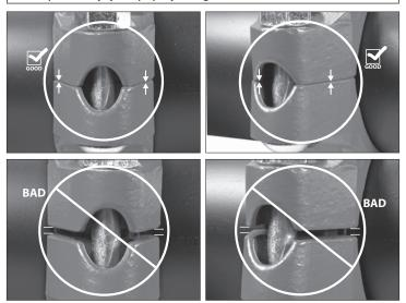
7. Visually inspect each bolt pad location at every joint to verify that metal-to-metal contact is achieved across the entire bolt pad section.
