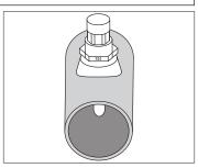
1. CHECK THE STYLE 923 OR 924: Verify that the "923" or "924" marking on the top hex nut is facing toward the curvature of the collar (along pipe axis), as shown above.
