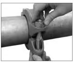
**3. INSTALL BOLTS/NUTS:** Install the bolts, and thread a nut finger-tight onto each bolt. **NOTE:** Verify that the oval neck of each bolt seats properly in the bolt hole.
