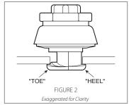
**5. POSITION STYLE 923 OR 924:** Shift the Style 923 or 924 to position the "heel" inside the pipe. **NOTE:** The heel shall be positioned, as shown in Figure 2 above, to ensure proper performance under operating conditions.
