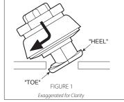
**4. INSERT STYLE 923 OR 924:** Align the "foot" of the Style 923 or 924 with the pipe. Tilt the "toe" into the outlet hole to insert the Style 923 or 924 (refer to Figure 1 above).
