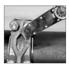
10. TIGHTEN NUTS: Using an impact tool or a standard socket wrench with a deep-well socket, tighten the nuts evenly by alternating bolt pad locations until the gaps are equal at all bolt pads. Verify that the oval neck of each bolt seats properly in the bolt holes. To complete the assembly, apply torque to each nut with a torque wrench. Refer to the "Assembly Torque Requirements" table on the following page and the "Torque Wrench Selection" section in this handbook.
