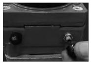
1. Remove the dust cap from the right side of the gear operator.
