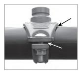
**6. INSPECT THE ASSEMBLY:** When the Style 922 is assembled correctly, the upper (outlet) housing, near the gasket, will not make metal-to-metal contact with the pipe. If there are gaps between the upper (outlet) housing's and lower housing's bolt pads, they shall be equal on both sides of the assembly.
