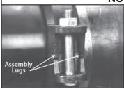
Victaulic Style 707-IJ Transition Couplings are designed with assembly lugs to ensure proper assembly of housings (NPS to NPS and JIS to JIS). These assembly lugs shall be on opposite sides for proper assembly.
