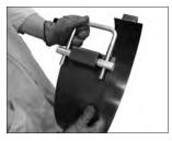
2. INSERT U-BOLT: Insert a U-bolt into the crossbar on both sides of the strap. The threaded ends shall protrude through the flat sides of the crossbars.
