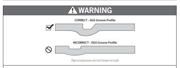
DO NOT attempt to assemble the Style W741 on pipe that is grooved with OGS roll sets.
