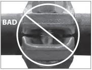
Visually inspect the bolt pad location at every joint to verify that metal-to-metal contact is achieved, in accordance with step 5.
