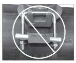
**NOTE:** Over-tightening one nut can cause damage to the threads and may cause the assembly to shift position, as shown to the left.
