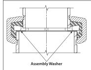
FOR VERTICAL INSTALLATIONS: An assembly washer is recommended to prevent smaller pipe from telescoping inside larger pipe in vertical installations (refer to graphic shown to the left). Contact Victaulic for details.
