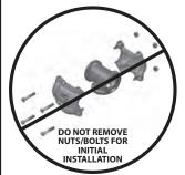
1. DO NOT DISASSEMBLE THE FITTING FOR INITIAL INSTALLATION: Victaulic® FireLock™ No. 102 and 104 Installation-Ready™ Fittings are designed so that the installer does not need to remove the nuts and bolts for initial installation. This facilitates installation by allowing the installer to directly insert the grooved end of mating components into the fitting.
