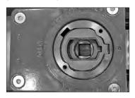
**3.** Turn the handwheel counter-clockwise. Verify that the valve is in the fully "OPEN" position by checking the position indicator on top of the stem, as shown to the left. The position indicator on top of the stem should be 90° from the correctly adjusted "SHUT" position.
