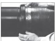
3. JOIN MATING COMPONENTS: Align the centerlines of the NPS and JIS grooved mating component ends and bring them to within the appropriate pipe-end separation dimension. Slide the gasket into position and center it between the groove of each mating component. NOTE: Verify that no portion of the gasket extends into the groove of either mating component and that the NPS side of the gasket is facing the NPS mating component.
