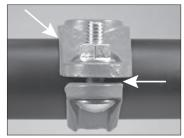
**6. INSPECT THE ASSEMBLY:** When the Style 912 is assembled correctly, the upper (outlet) housing, near the gasket, will not make metal-to-metal contact with the pipe. If there are gaps between the upper (outlet) housing's and lower housing's bolt pads, they shall be equal on both sides of the assembly.
