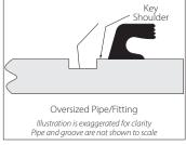
When the OD of the pipe or fitting exceeds the maximum tolerance, engagement of the housings' key sections is increased to the point that the shoulder can grip onto the pipe and can result in reduced linear or angular movement. Under these conditions, metal-to-metal bolt pad contact may not be achieved, the gasket may become extruded, the working pressure of the joint may be reduced, and gasket life may be reduced.
