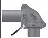
**5b. COMPLETELY TIGHTEN NUT AT INSIDE LOCATION:** Completely tighten the nut at the inside location until metal-to-metal contact occurs at the bolt pads. Verify that the fitting's keys still engage the grooves completely and that the oval neck of the bolt seats properly in the bolt hole.
