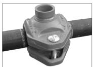
**4. ASSEMBLE JOINT:** Assemble the joint by inserting the grooved end of a mating component into each opening of the coupling. The grooved mating component ends shall be inserted into the coupling until contact with the pipe stop of the gasket occurs.
