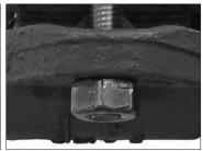
**7. INSTALL BOLT AND NUT:** Install the bolt, and thread a nut onto the bolt. **NOTE:** Verify that the oval neck of the bolt seats properly in the bolt hole. DO NOT tighten the nut completely. The bolt pads need to be set at a gap for reinstallation of the coupling. The nut should be flush with the top of the bolt to provide the proper gap.
