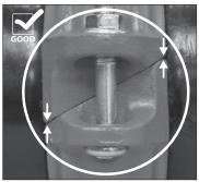
PROPERLY ASSEMBLED JOINT **BOLT PADS WITH EQUAL, NEUTRAL** OFFSETS AT THE BOLT PADS
