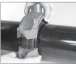
**5. INSTALL UPPER HOUSING:** Install the upper housing over the gasket. Verify that the housings' keys engage the grooves completely on both mating components. Inspect the outlet opening to verify that the outlet neck of the gasket is positioned properly in the upper housing.
