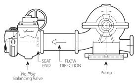
Series 377 Vic-Plug Balancing Valves shall be installed with the seat upstream (closest to the pump discharge)
