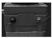
2a. Loosen the hex lock nut (counterclockwise) located on the right side of the gear operator.
