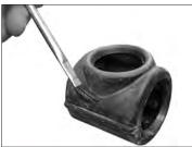
**5. FOR REASSEMBLY OF STYLE 118 OUTLET COUPLINGS, LUBRICATE GASKET:** Apply a thin coat of a compatible lubricant to the three gasket sealing lips and exterior. Refer to the "Lubricant Compatibility for Gaskets" table on page 34.
