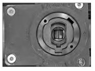
**3.** Verify that the valve is in the fully "SHUT" position. The fully "SHUT" position can be verified by removing the indicator cap from the top of the gear operator and checking the position indicator on top of the stem, as shown to the left.
