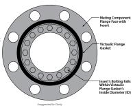
• When mating two Style 741, 841, 743, 744, or 341 Flange Adapters, the Victaulic Flange Washer shall be placed between the two Victaulic Flange Adapters with the hinge points staggered.
