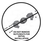
1. DO NOT DISASSEMBLE THE FITTING FOR INITIAL INSTALLATION: Victaulic® FireLock™ No. 101 and 103 Installation-Ready™ Fittings are designed so that the installer does not need to remove the nuts and bolts for initial installation. This facilitates installation by allowing the installer to directly insert the grooved end of mating components into the fitting.
