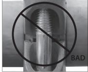
5. Visually inspect each bolt pad location at every joint to verify that proper assembly is achieved (refer to the "NOTICE" above for Style HP-70 Couplings in 6 – 12-inch/DN150 – DN300 sizes).
