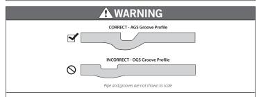
DO NOT attempt to assemble Style W07/LW07, W77, or W89 AGS Couplings on pipe that is direct-grooved with OGS roll sets.
