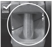
PROPERLY ASSEMBLED JOINT METAL-TO-METAL CONTACT AT ANGLED METAL-TO-METAL CONTACT AT ANGLED **BOLT PADS WITH EQUAL, NEUTRAL** OFFSETS AT THE BOLT PADS
