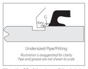
When the OD of the pipe or fitting is below the minimum tolerance, engagement of the housings' key sections is lowered considerably. THIS RESULTS IN REDUCED WORKING PRESSURE FOR THE JOINT.
