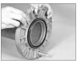
**6. INSTALL STYLE 441:** Install the hinged Style 441 around the grooved pipe end. Verify that the key section of the housings engages with the groove in the pipe end.
