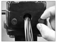
**2.** Remove the dust cap from the right side of the gear operator.
