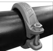
**5. ASSEMBLE JOINT:** Assemble the joint by inserting the grooved end of a mating component into each opening of the coupling. The grooved mating component ends shall be inserted into the coupling until contact with the center leg of the gasket occurs.
