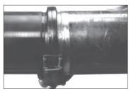
4. INSTALL HOUSINGS: Install the housings over the gasket with the assembly lugs on opposite sides. Verify that the larger openings of the housings (marked NPS) face the larger mating component (NPS side) and that the housings' keys engage the grooves completely on both mating components.
