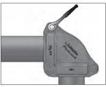
7. COMPLETELY TIGHTEN NUT AT FIRST OUTSIDE LOCATION: Go back and completely tighten the nut at the first outside location to confirm metal-to-metal contact at the bolt pads.
