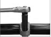
5. TIGHTEN NUT: Using an impact tool or a standard socket wrench with a deep-well socket, tighten the nut.
