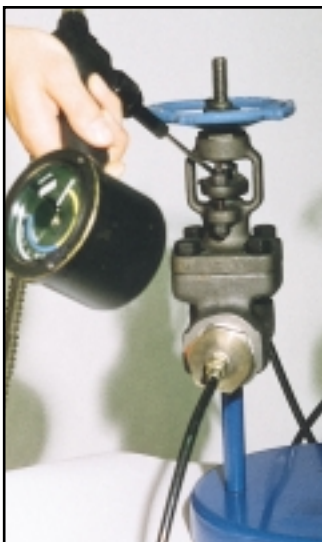
Velan API 602 Class 800 forged steel gate valve.
