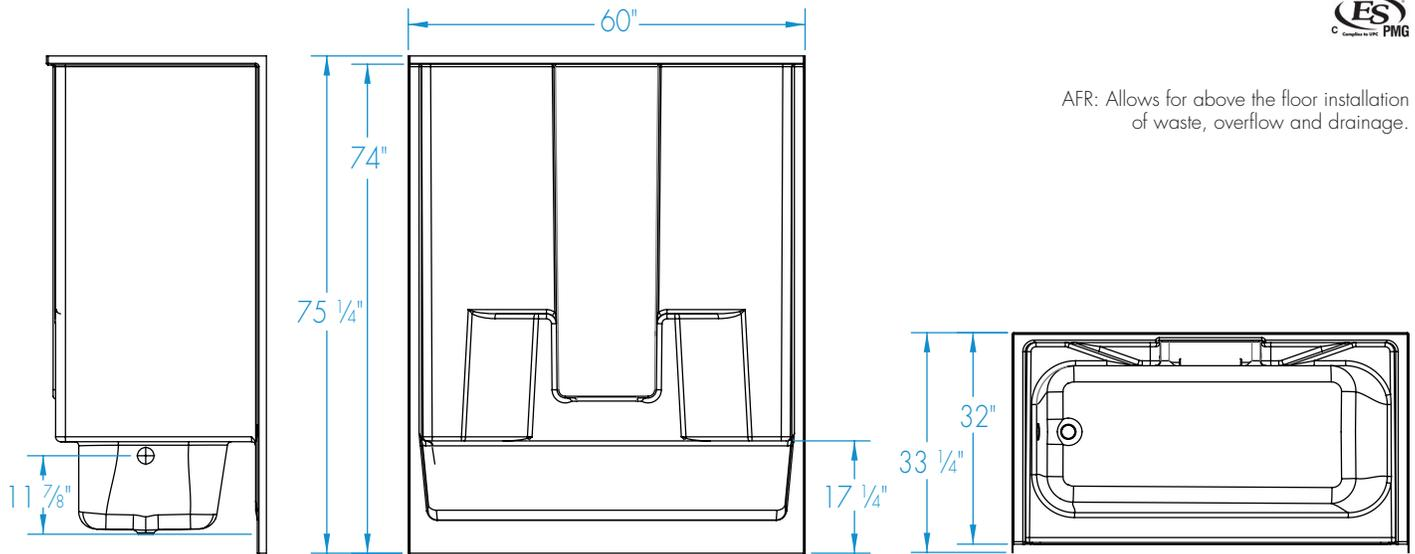
**FEATURES** lbs Dimensional Tolerance  $\pm 3\%$ . Dimensions needed for site preparation should be measured from the unit. Aquatic assumes no responsibility for preparatory work.
