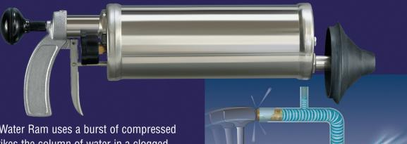
The Kinetic Water Ram uses a burst of compressed air, which strikes the column of water in a clogged pipe. The resulting shock wave, called Kinetic Energy, hits the stoppage at a speed of approximately 4,700 feet per second, quickly clearing the blockage and flushing waste particles away.
