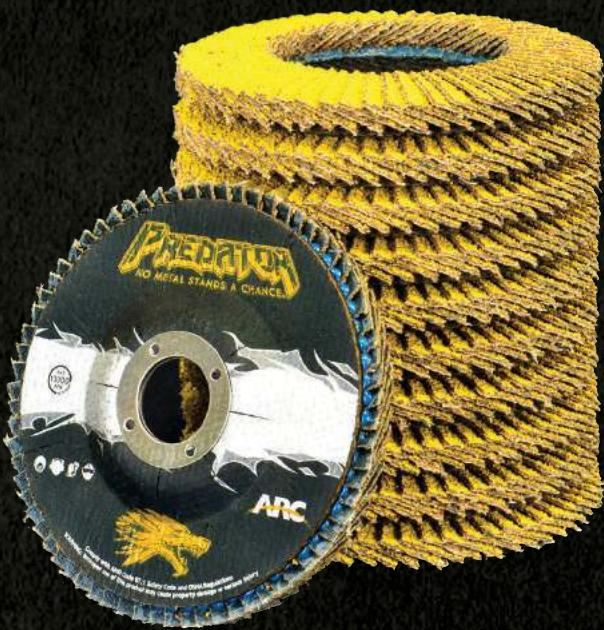
Hard Edge discs have a shape similar to our Type 29, or angle faced discs, but are engineered for extremely fast material removal using a reduced amount of pressure. This is accomplished by compressing the outside rim of the flaps to eliminate flexing during the grinding process.
