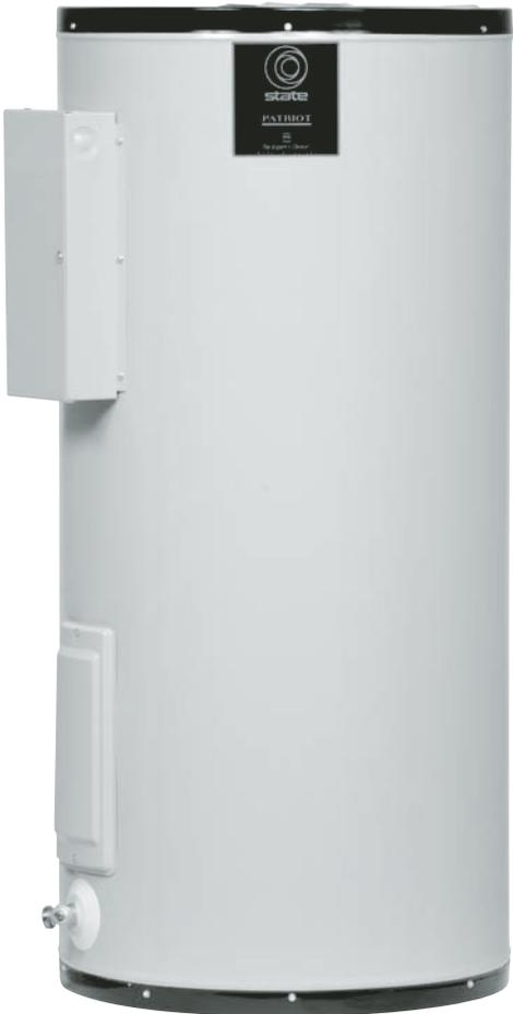
Designed for use as recovery heaters for light-duty hot water supply service. Patriot™ PCE water heaters are available with tank capacities from 6 through 119 gallons. They can be installed for non-simultaneous and single element operation (maximum input up to 6 KW), or for simultaneous dual-element operation (maximum input up to 12 KW).
