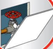
**Align panel's inside ledge with bottom of opening, then push panel against wall. To remove, simply pull out at opposite corners.**
