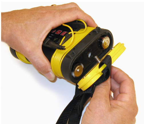
Figure 4 – Removing the Battery Cover
