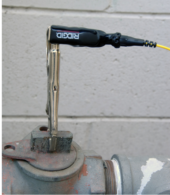
Figure 8 – Alternative hookup method
