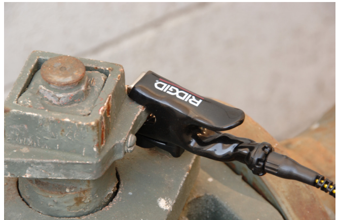
Figure 6 – Connecting the ST-305 using the clip
