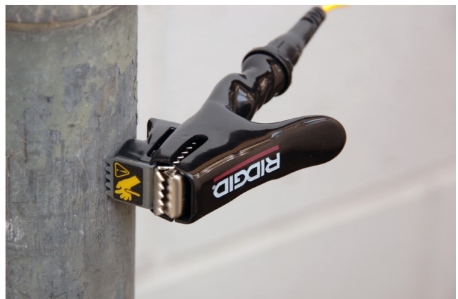
Figure 7 – Connecting the ST-305 using the magnet
