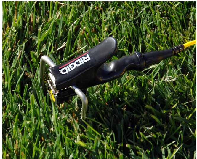
Figure 5 – Connecting the ST-305 Ground Stake
