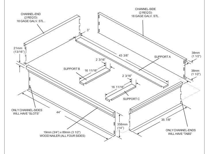
Figure 4. BAYCURB050A Component Drawing
