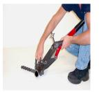
2. Wrap chain around pipe and engage nearest pin in upper jaw hooks.
