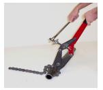
4. Place ratchet on head of drive screw and operate clockwise until pipe snaps off. If pipe has not cut before jaw wheels touch, turn counterclockwise until next pin can be engaged in jaw. Repeat Step 4.
