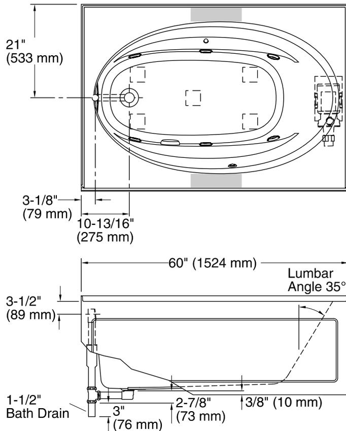
No change in measurements if connected with drain illustrated. (K-11677)
