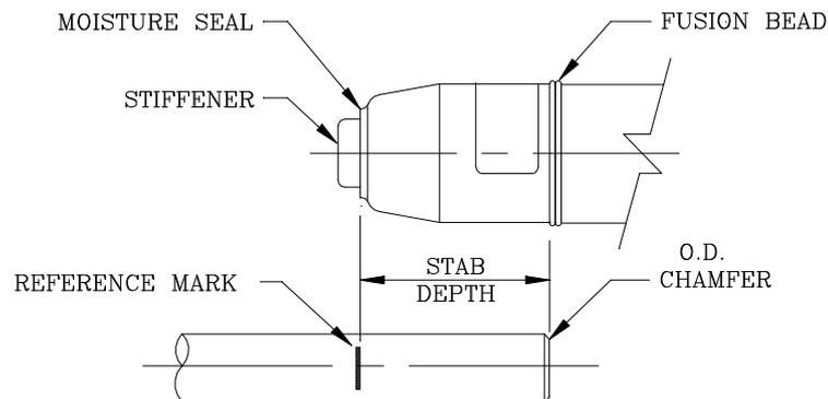
6. Stab the tube into coupling until it bottoms. The reference mark will be:
