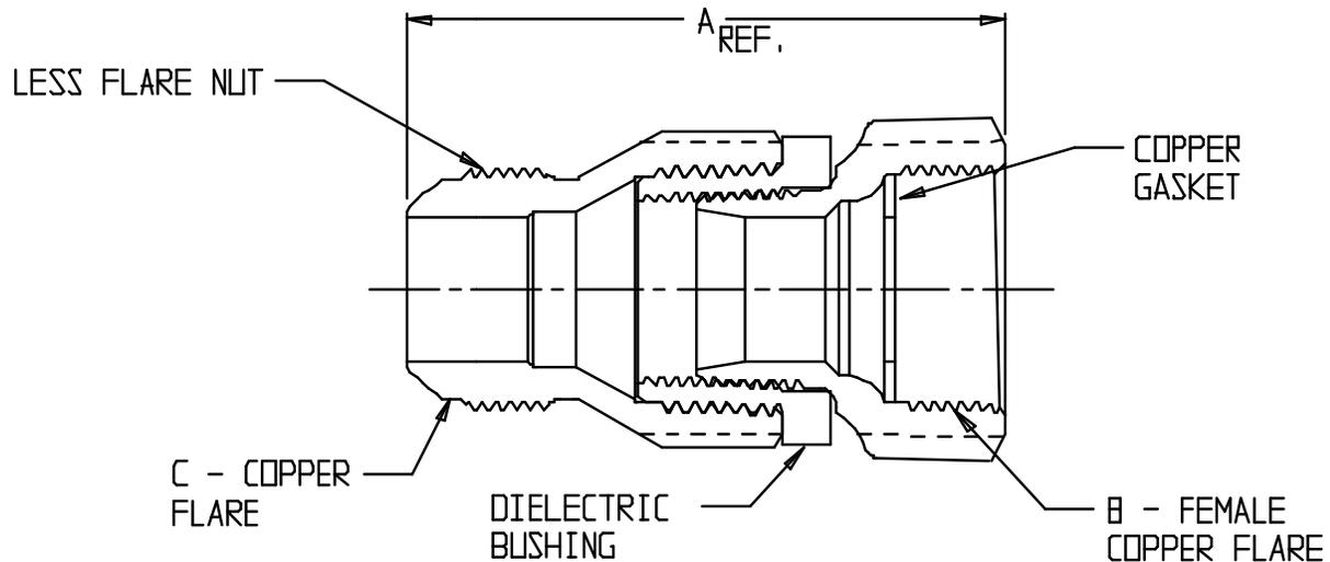
NOTE: ACTUAL LENGTHS WILL VARY DUE TO ASSEMBLY OF INSULATOR.
