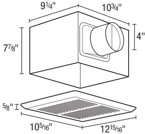
Acceptable for use over tub or shower when installed in a GFCI protected branch circuit.
