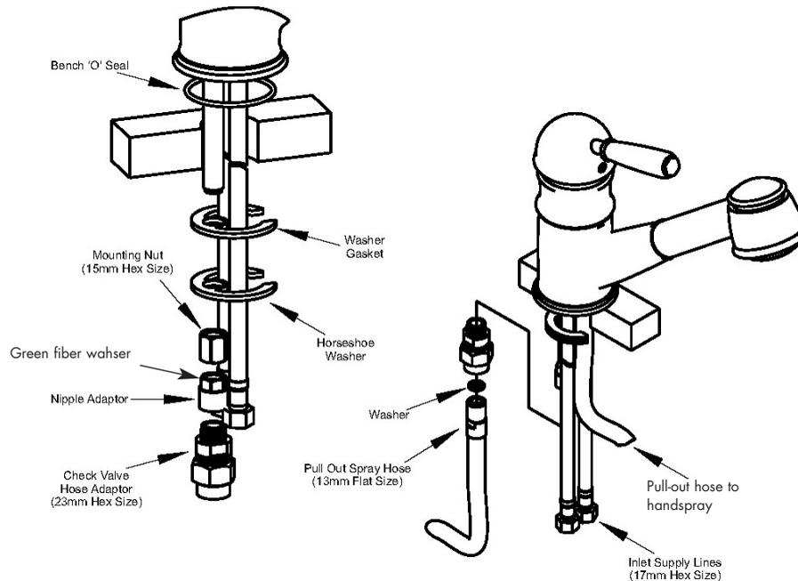
**Note: This mixer fits a maximum bench thickness of 2-1/2" and has a 90° spout arc.**
