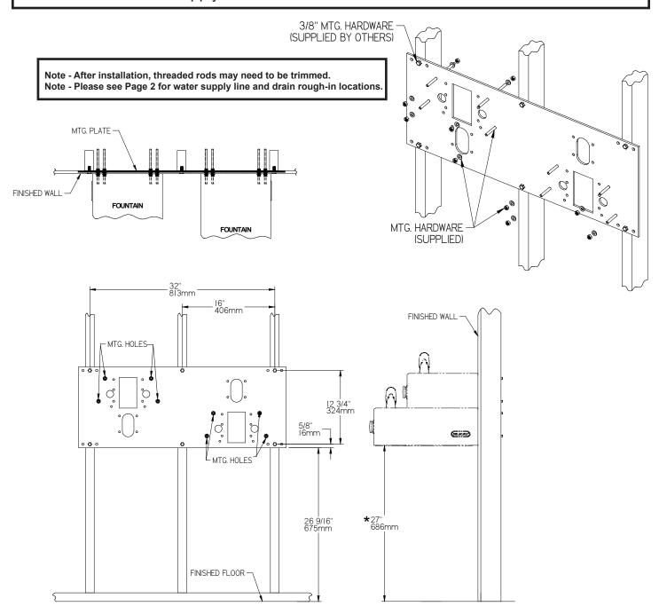
\*ADA REQUIREMENT NOTE - AFTER INSTALLATION, THREADED RODS MAY NEED TO BE TRIMMED
