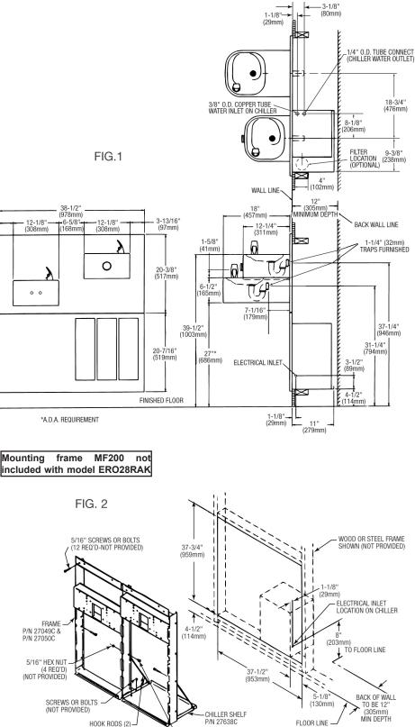
BOLT FRAMES TOGETHER -WITH 5/16" X 3/4" (19mm) BOLTS (4 REQ'D-NOT PROVIDED)
