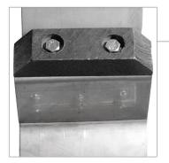
Each band is lined with EPDM liner attached to the band. Runner surface is comprised of UHMW polymer for abrasion resistance and a low coefficient of friction. The runners and risers are attached at appropriate positions to properly support the carrier within the casing in order to ease installation.
